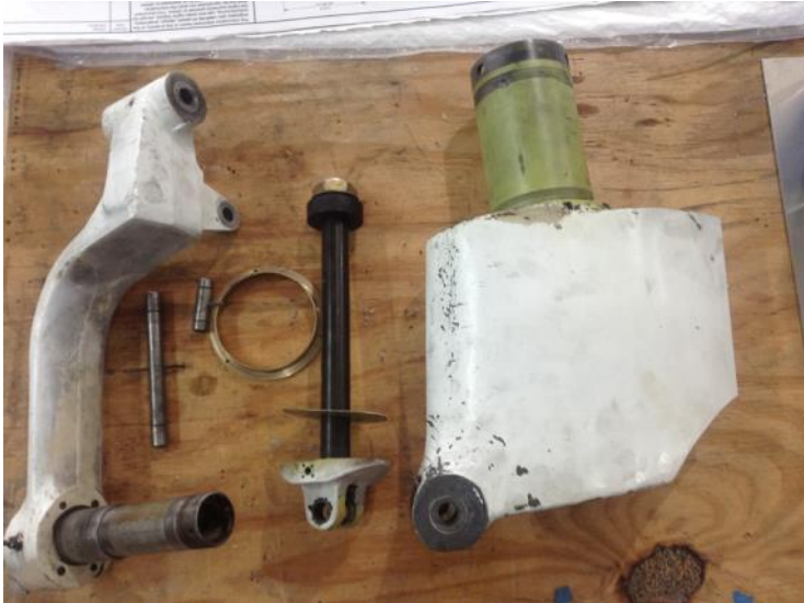
Photo 1: Nose strut of a Musketeer. Several different metals. The large white fairing is magnesium.
