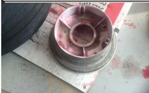
In this photo, the dye has been sprayed on, allowed to penetrate, cleaned off, and developer (white powder) is drying. A crack will show up as a red line.
