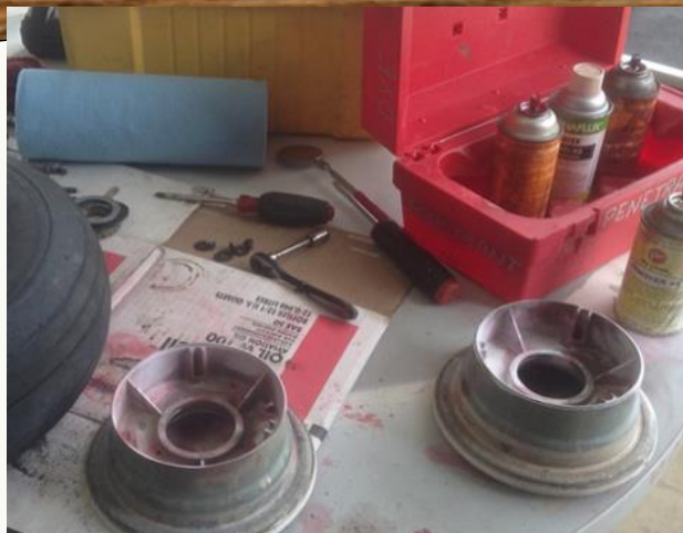
Here is a Cleveland 6:00 DMB. The left half in the photo has developer already on it. The right half is cleaned and ready for the dye penetrant process.
