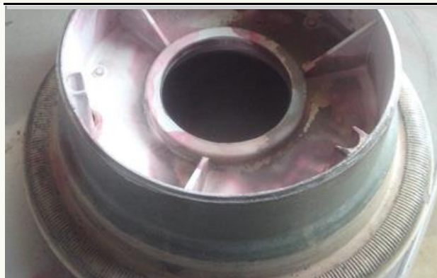
This last photo shows the developer mostly dry. No cracks were found this time.
