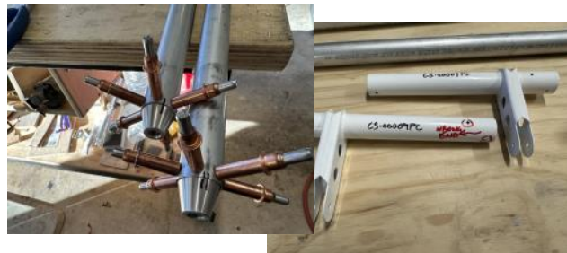
Zac Morton working worked on aileron push-rods and discovered a manufacturing error in one of his torque tubes
