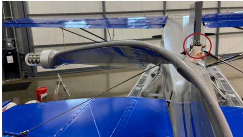
A Piper PA-12 on floats became nearly impossible to control after the airplane's rudder post fractured above the upper hinge (circled) on June 8, 2020, causing the top of the rudder to fold over in flight. NTSB photo.
