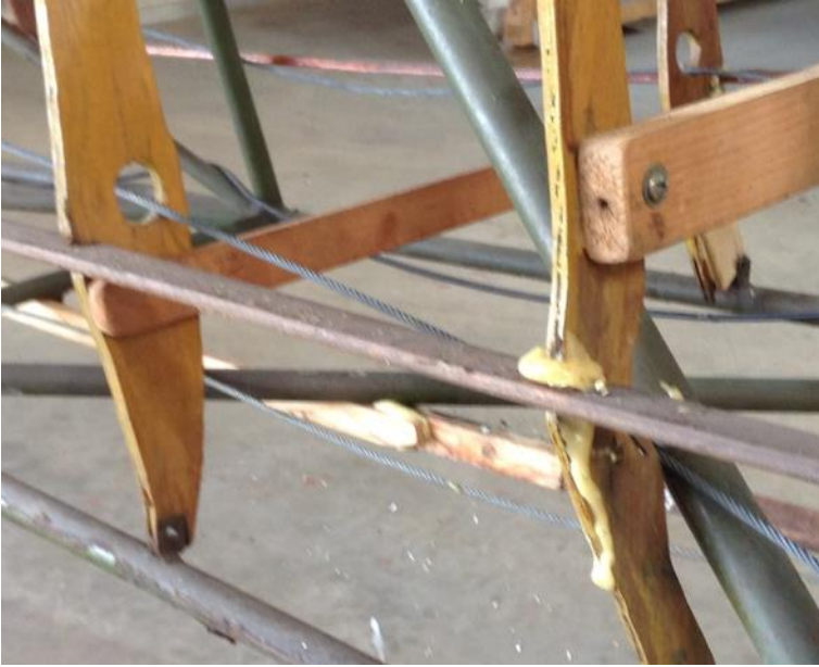
Photo 2: The foamy yellow stuff is urethane glue, aka Gorilla Glue. Very few types of glue are approved for aircraft use and this is not one of them.
