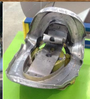
Photo 3: Abused landing light housing.
