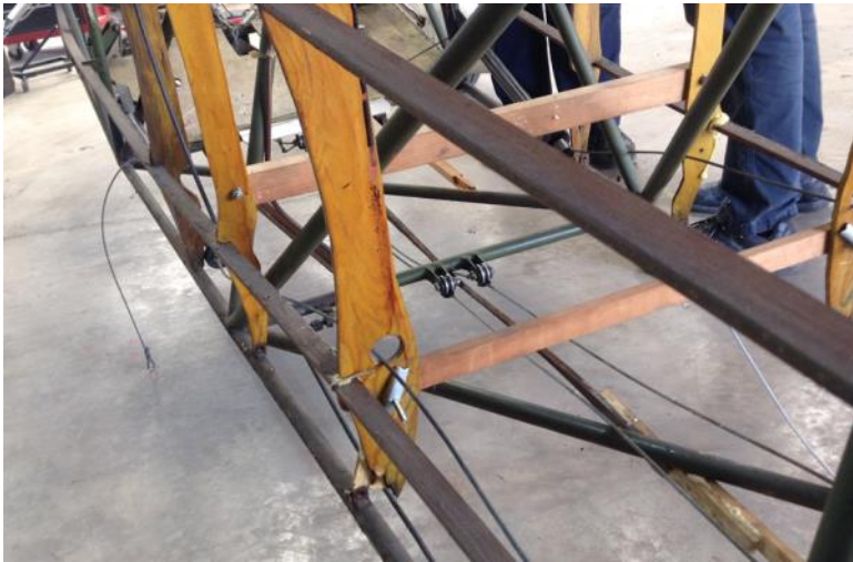
Photo 2: The foamy yellow stuff is urethane glue, aka Gorilla Glue. Very few types of glue are approved for aircraft use and this is not one of them.
