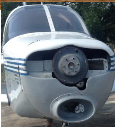
Photo 2: Missing landing light – Hint: it was in the oval hole beneath the
