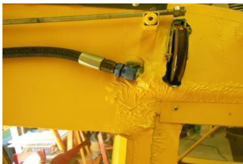
Photo 1. Gasoline damaged finish.
