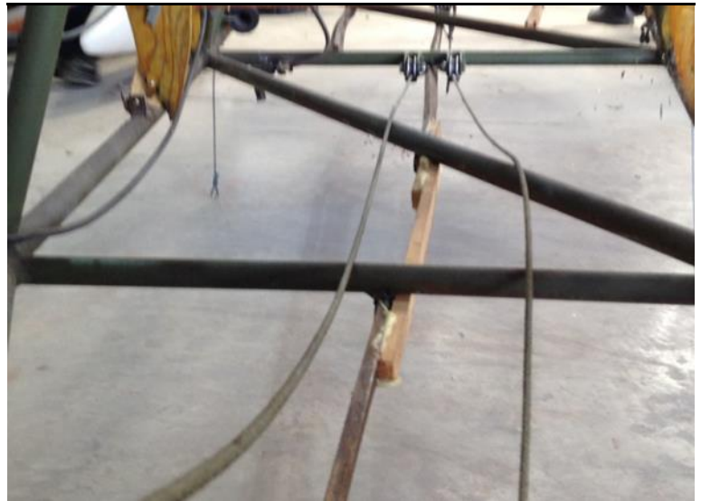
Photo 5: The belly stringer has been spliced with pine and urethane glue.
