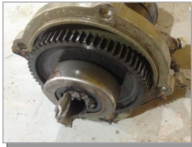
Photo 1: Starter pinion gear destroyed by engine kickback
