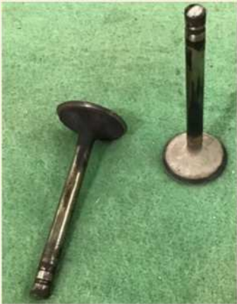
Photo 3: Continental A-65 exhaust valves.
