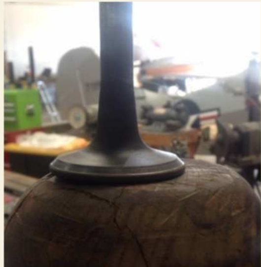
Photo 9: Cupped valve face.
