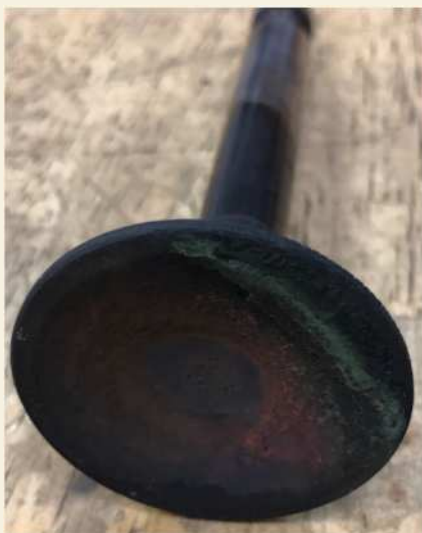
Photo 8: Badly damaged exhaust valve
