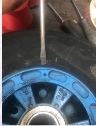
Photo 10: Twist don't pry the screwdriver. A bit of penetrating oil helps.
