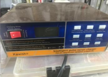
Photo 8: Smart Charger. This little gem does 12 and 24 volts. It self-adjusts current and can even do limited battery cell repair. As an added bonus, the controls have Cyrillic and English labels.
