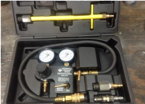
Photo 1: Compression test kit with compression tester extension
