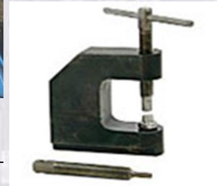
Photo 11: Brake rivet tool. Threaded style not the impact style.
