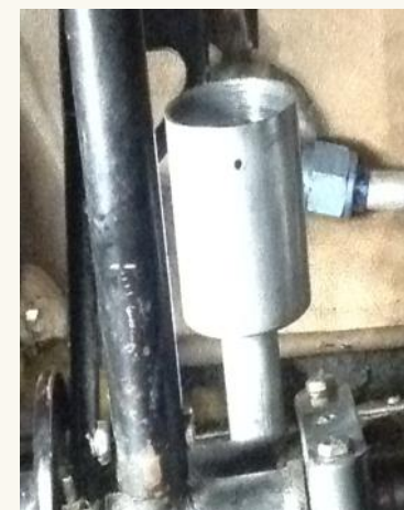
Photo 2: Cessna Master Cylinder in situ with top and insides removed.
