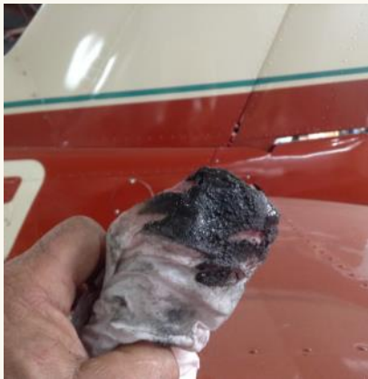
Photo 3: Dirt swabbed out of the fluid cup. The sludge was about \frac{3}{4} inch deep.
