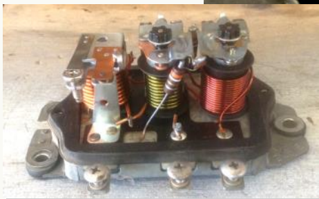
Figure 4: Electromechanical voltage regulator outside and inside.
