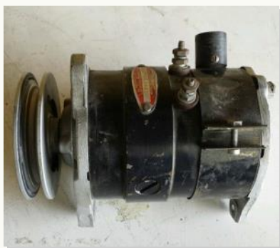
Figure 1: A Delco-Remy 20 amp generator. The tube and shroud are to direct cooling air into the housing.
