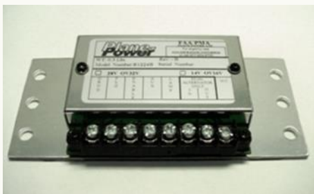
Figure 5: Solid State Voltage Regulator. Photo by Aircraft Supply company.
