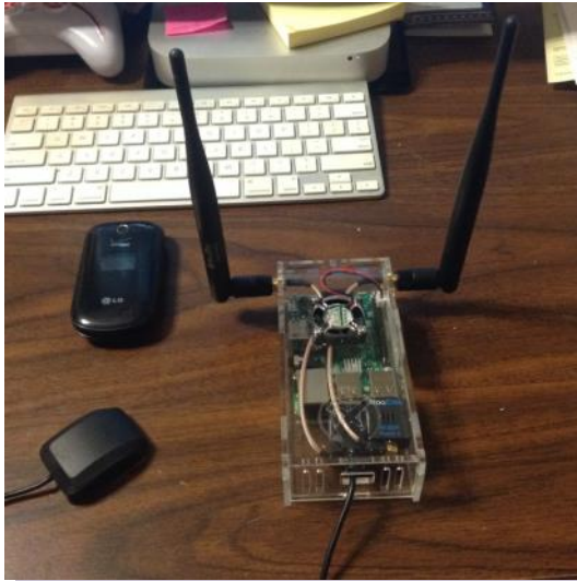
Photo 3: Assembled! Everything plugs in or screws in. The only hassle was that the power cord I wanted to use would not fit through the hole in the case. That was easily fixed with a needle file.
