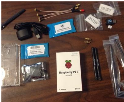
Photo 1: Components of ADS-B Receiver Kit. The clear plastic case is at the left. At the right are both hi and low gain antennas but only one or the other set is required.
