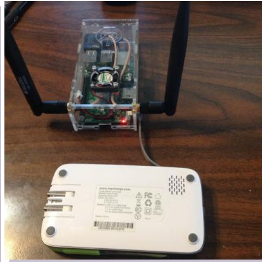
Photo 4: A portable device charger powering the ADS-B receiver
