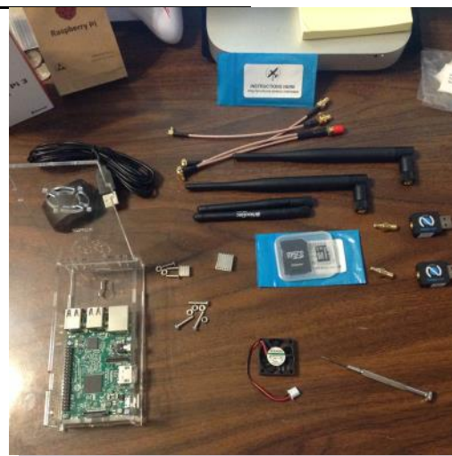
Photo 2: Beginning assembly. The Pi is in the case. Technically speaking, unless you are over-clocking the cpu, the metal heat sinks should be sufficient and the little muffin fan can be left off.
