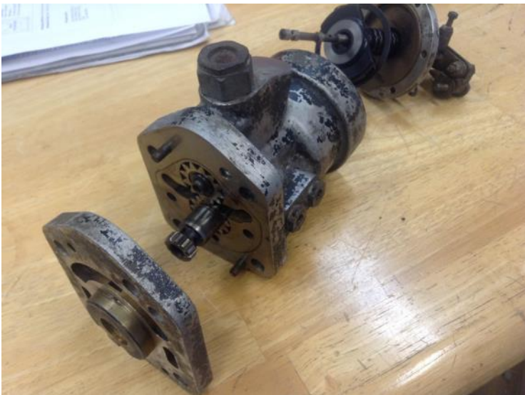
Photo 2: Oil pump neatly nested inside the propeller governor. The engine's accessory drive turns the small gear seen at the lower left.
