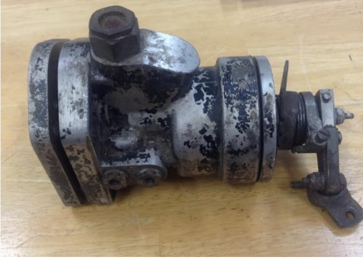
Photo 1: Typical, general aviation style propeller governor.
