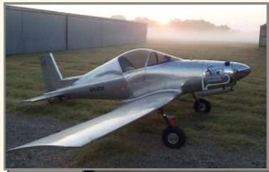
remained from the original modified Hummel. He designed longer, wider tapered wing panels that attach at the fuselage. Bruce says that saves as much as 6 months of center wing construction. He used center-section mounted spring aluminum gear in place of the original stiff tube struts for better ground handling and ease of construction.
