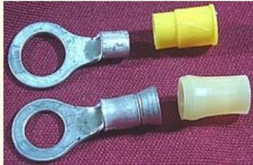
Insulating sleeves are removed here for clarity. Upper terminal is general purpose/automotive use. Lower terminal is aircraft grade. Photo Credit: Sacramento Sky ranch
