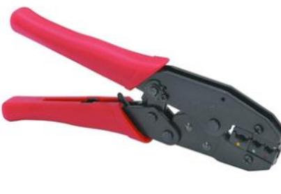
Good tool. Ratcheting crimp tool with jaw openings for red, blue and yellow terminals.
