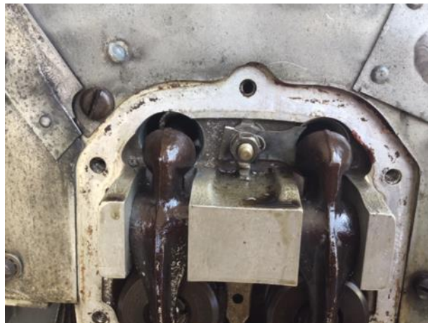
Figure 4: Rocker cover removed from O-360 cylinder.
