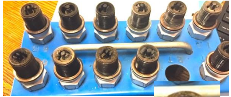
Figure 5: Fouled spark plugs
