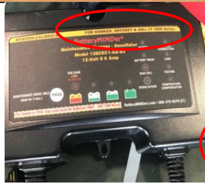
Photo 3: For Hawker, Odyssey, and Gill 7000 VRLA batteries.
