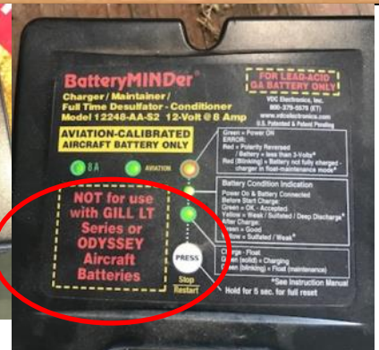
Photo 4: For General VRLA Batteries but NOT for Gill or Odyssey.
