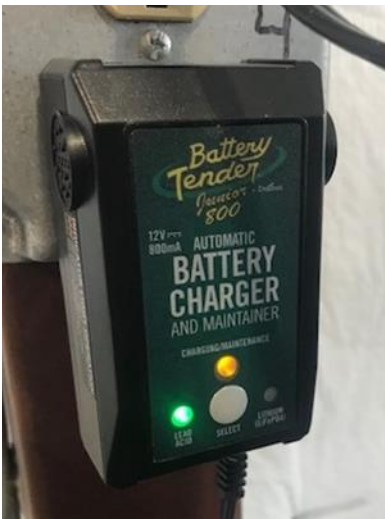
Photo 1: Smart charger good enough for a computer battery and will work OK for a VRLA on your plane. However, it is not optimum.
