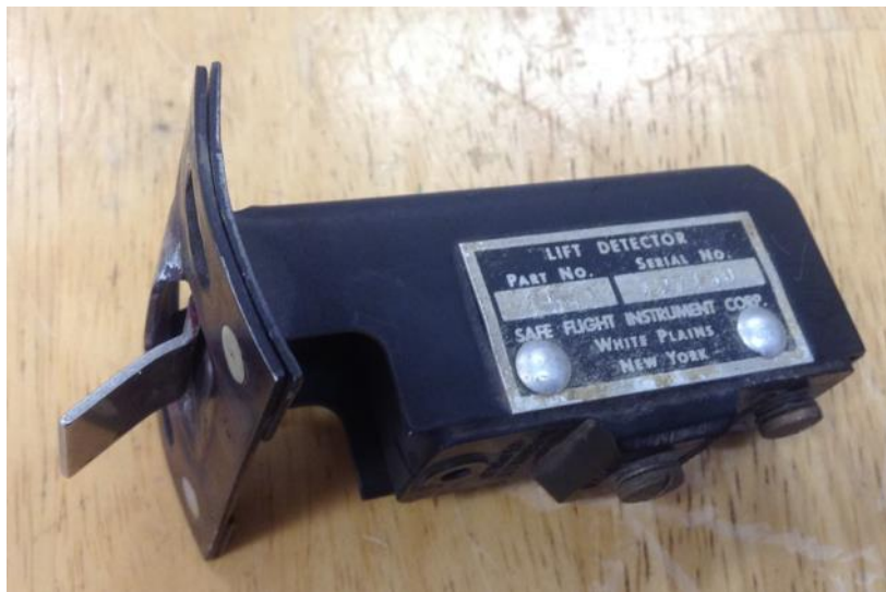
Lift Detector made by Safe Flight Instrument Corporation
