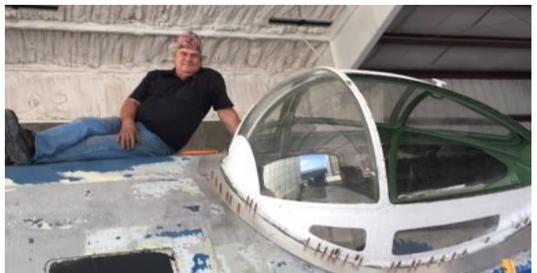
This is our own Jake White, A&P, IA with the first of his hand-crafted bubbles on a PBY Catalina. This is a fully functional, exact reproduction on a plane being restored for a museum display. This takes a lot of skill — and a lot of patience!
