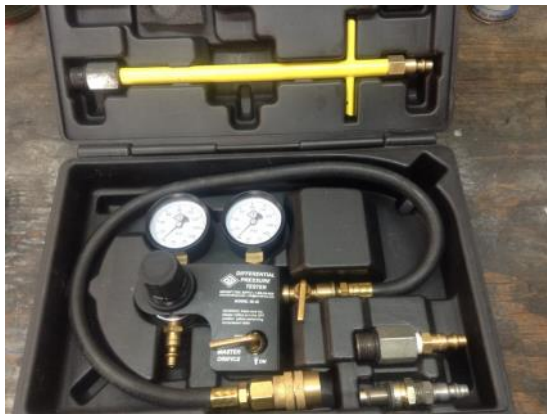
Compression test kit with compression tester extension
