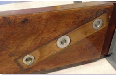
Bushings in the spar of a Citabria
