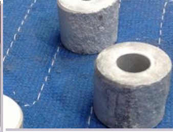
Bushings removed from the spar
