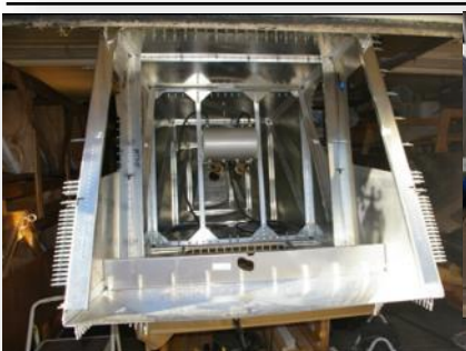
Header Tank and Fuel Pumps
