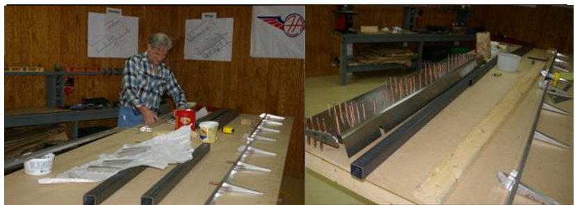
Fabrication of the Flaperons
