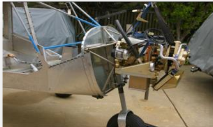
Viking Engine Install to Firewall
