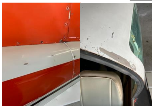
Photo 7: Minor peeling paint.
