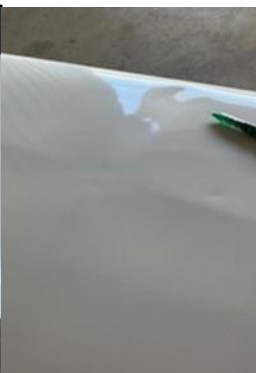
Photo 13: Dent in horizontal stabilizer.
