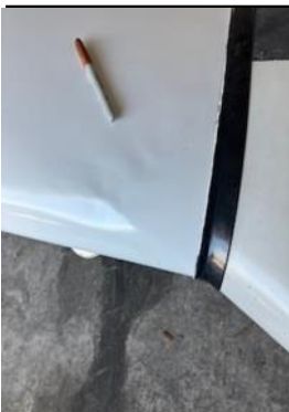
Photo 11 and 12: Dents in top skins near wing root.
