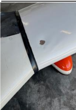
Photo 11 and 12: Dents in top skins near wing root.
