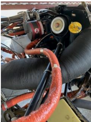
Photo 1: Clean engine. Good fire sleeves
