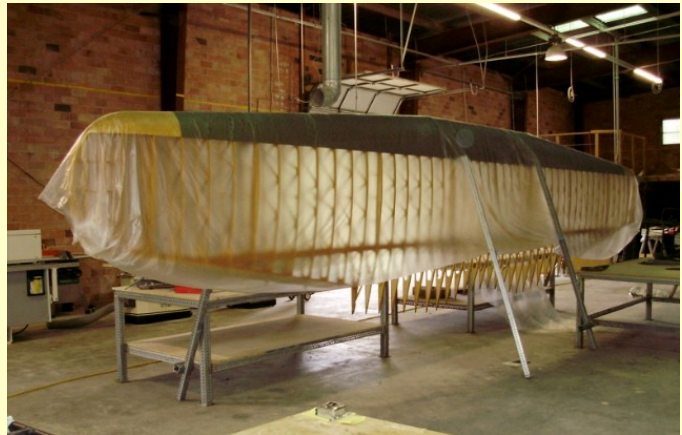
Upper wing ready to cover
