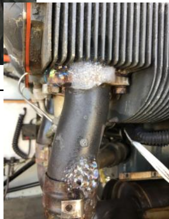
Photo 6: Bubbles at a pipe coupler and a different exhaust flange.
