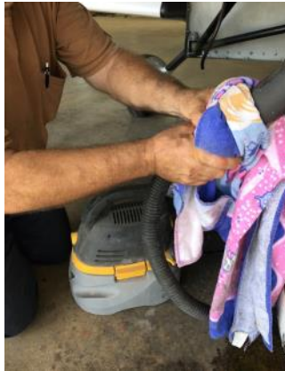
Photo 4: Pressurizing the exhaust system via shop vac.
