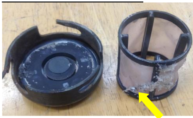
Photo 2: Dirty fuel filter. Note the piece of rivet.
