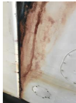
Photo 9: Old fuel stain along wing trailing edge.
