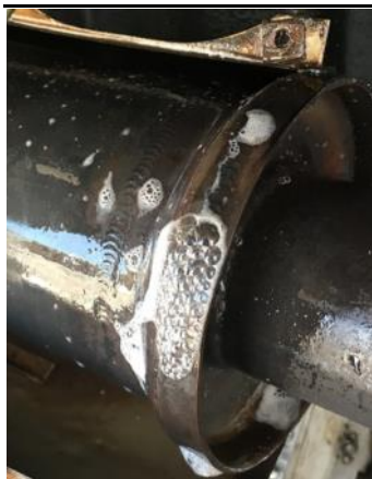
Photo 7: Bubbles at the end of the muffler.
