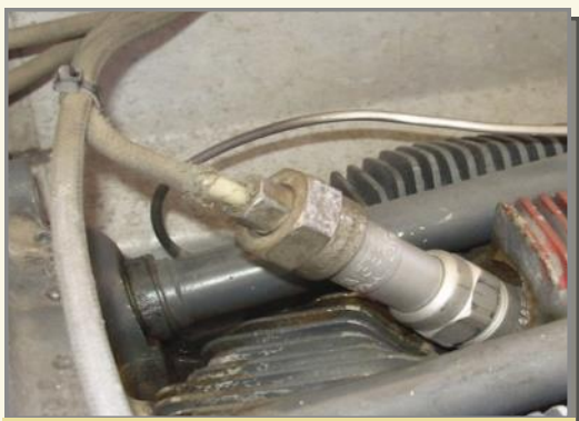
Frayed ignition shield wire exposes soft silicone
