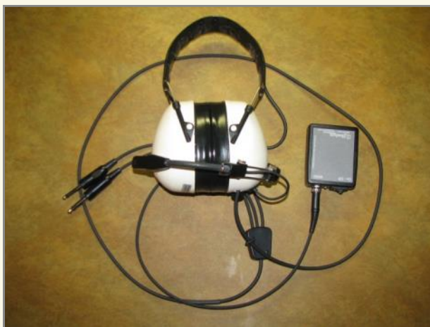
Figure 1. Peltor 7004's converted to ANR
