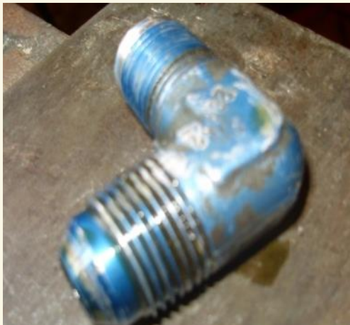
AN elbow – This side appears to be OK
