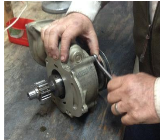
Photo 1: Opening the 90-degree drive adapter. The starter mounts on the flange behind the mechanic's right hand. The gear visible at the left engages the other accessory gears. The pulley at the right drives the alternator belt.
