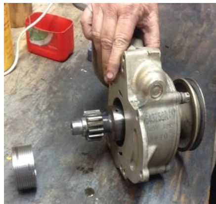
Photo 2: Half of the helical spring is on the workbench. The remainder of the spring is still inside the drive adapter body. Some of the drive shaft is showing below the mechanic's index finger.
