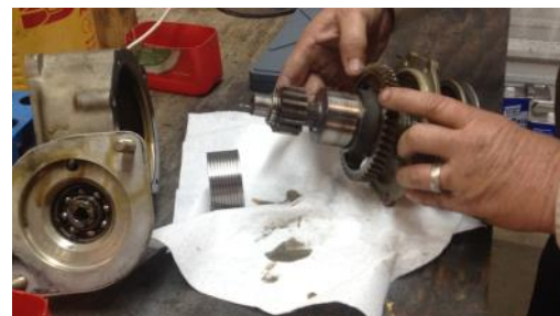
Photo 5: The starter motor mounts to the flange on the piece at the left of the photo. Notice the large ball bearing. The worm gear drives the round gear that is under the mechanic’s left index finger. The round gear is attached to the spring. Half of the spring is on the table, the other half is still on the drive shaft. The drive shaft is the shiny cylinder under the mechanic’s right thumb.
