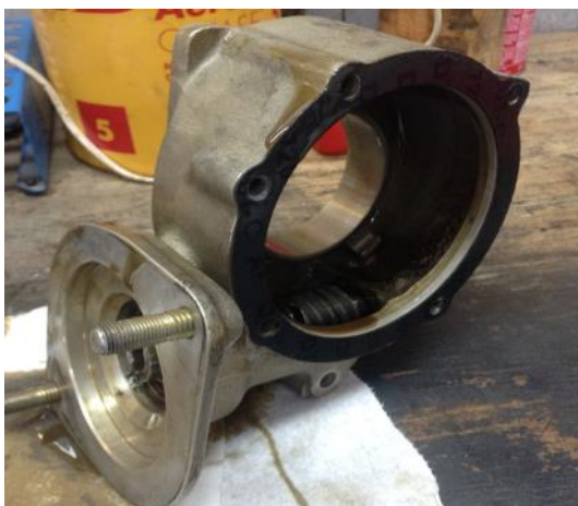
Photo4 : This is the drive adapter body further disassembled. The starter mounts on the flange at the left of the photo. The worm gear driven by the starter is visible in the body.
