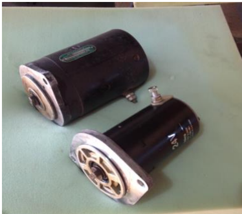
Photo 3: Prestolite starter upper left, TCM compact starter lower right.
