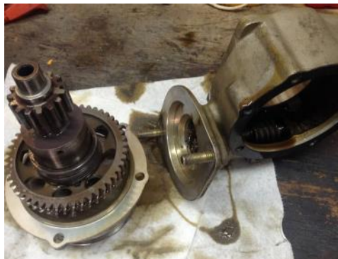
Photo 6: A close up of the drive adapter components. If the 90-degree drive were assembled, the large gear and cover plate would be at the lower left on the adapter body with the small gear protruding toward the upper center of the photo. The starter motor mounts to the flange in the center of the photo.
