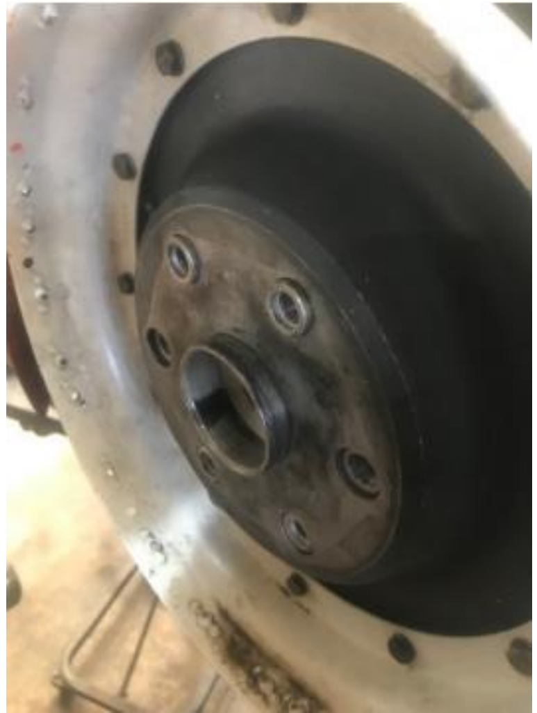
Photo 3: Orientation of flywheel, crankshaft and back shell is critical
