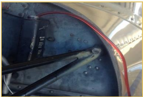
Plastic tube in a Piper brake reservoir. Note that Cessnas generally use two brake reservoirs mounted at the pilot's brake pedals.
