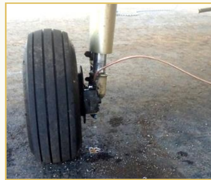
As you pump the brakes the air bubbles travel upward to the reservoir and escape to atmosphere.
