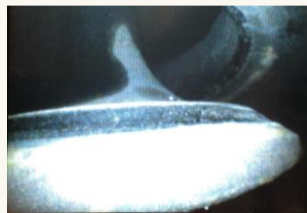
Photo 5: Here the exhaust valve is unseated. The valve stem is at the top of photo. Exhaust gas has burned a white streak up one side of the stem showing that the corresponding edge of the valve is not fully seating.
