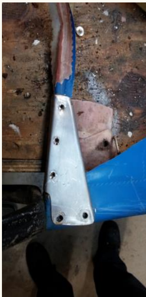
Photo 1: Fabric removal is underway. You can see where the stainless steel gusset had been riveted on
