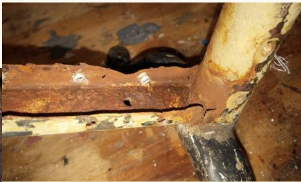
Photo 2: Rudderpost is the vertical tube on the right. The tail wheel steering arm is at lower right. The bottom rudder rib is literally rusted off.
