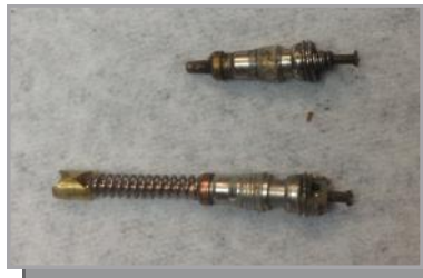
Photo 3: Two styles of Schrader valve, they don't last forever.
