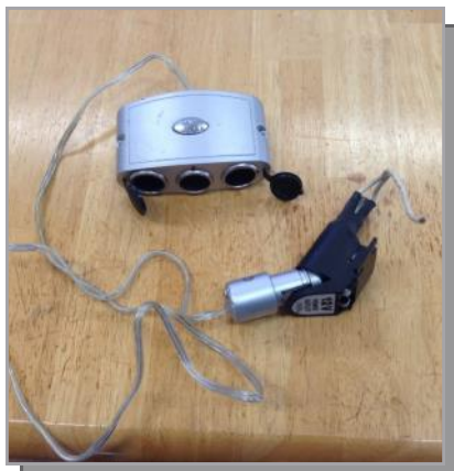
Photo 1: Wiring removed from a small, certified airplane. It was overloaded and the non-approved wire was giving off toxic fumes.
