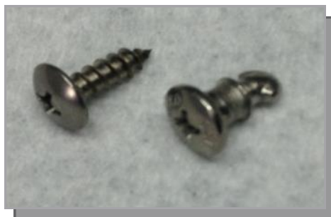
Photo 4: To the unwary, a Southco 1/4 turn fastener looks like a Phillips head screw
