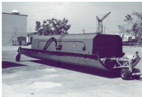
A ferry fuel tank for the B-57 on the upper half of the bomb bay door ready for installation.
