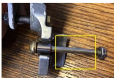
Photo 2: The downlock pin is actually a clevis bolt and roller/spacer shown here in the downlock hook.
