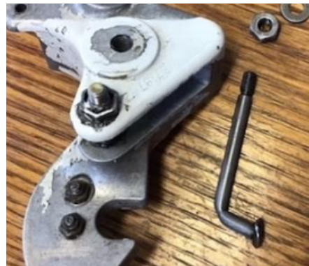
Photo 3: Bent Downlock Pin
