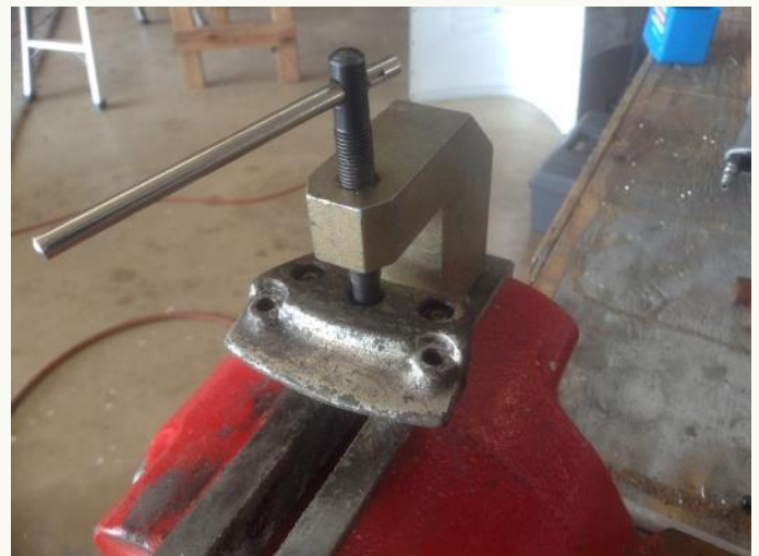
Photo 9: Setting a rivet.
