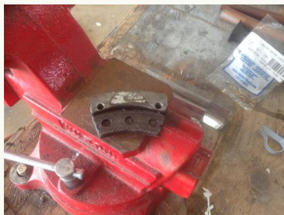
Photo 2: Brake pad riveted to a back plate showing plenty of pad life remaining.
