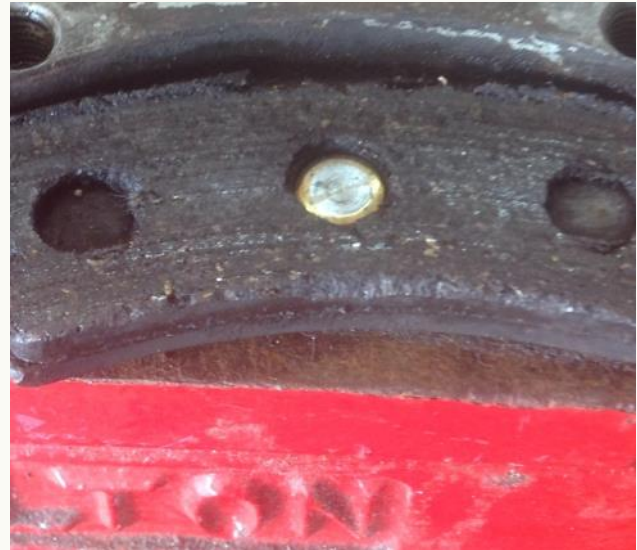
Photo 13: The manufactured head of the same rivet shown in photo 12. The manufactured head is recessed as deep as it can go.
