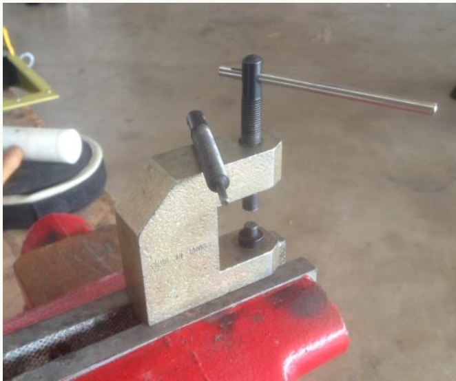
Photo 3: Good brake rivet tool. The rivet setting die in in the tool and the removable anvil is in place. The pin press die is resting on top.
