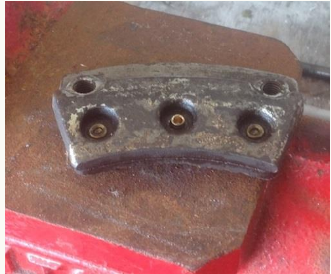
Photo 8: Rivet inserted and ready to be set.
