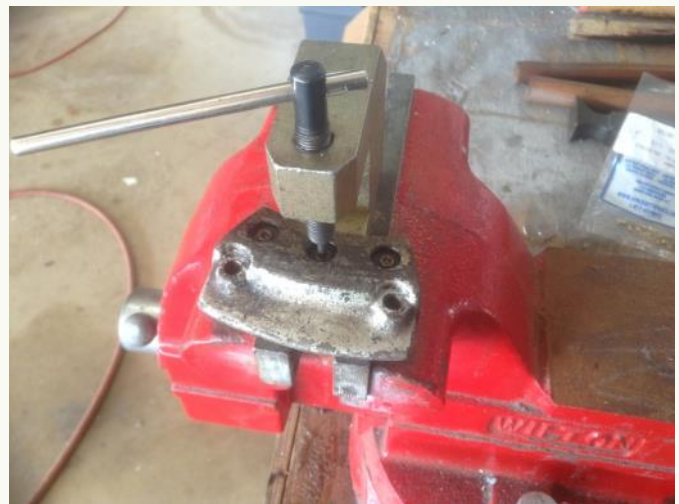
Photo 5: Rivet being pressed out.
