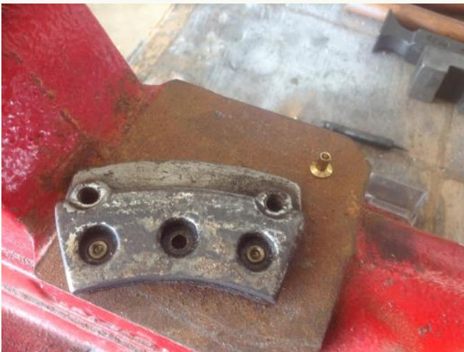
Photo 7: New brake rivet and a backing plate/pad assembly.
