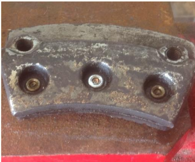
Photo 12: A new shop head on rivet. The rivet should not be able to move.
