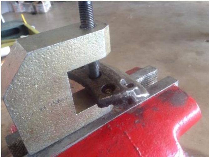
Photo 10: Another look at a rivet being set.
