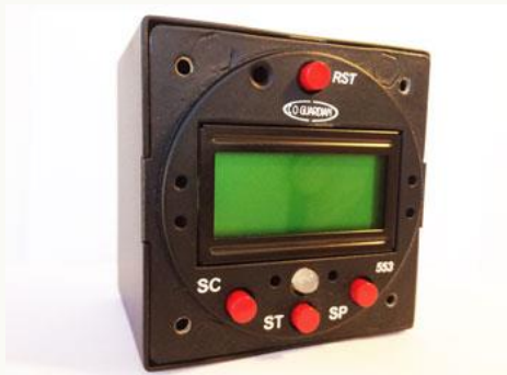
This sensitive CO detector also is a clock/timer/stopwatch and will alert if the cabin altitude exceeds safe no-oxygen levels. http://www.guardianavionics.com/aero553-101-001.html
