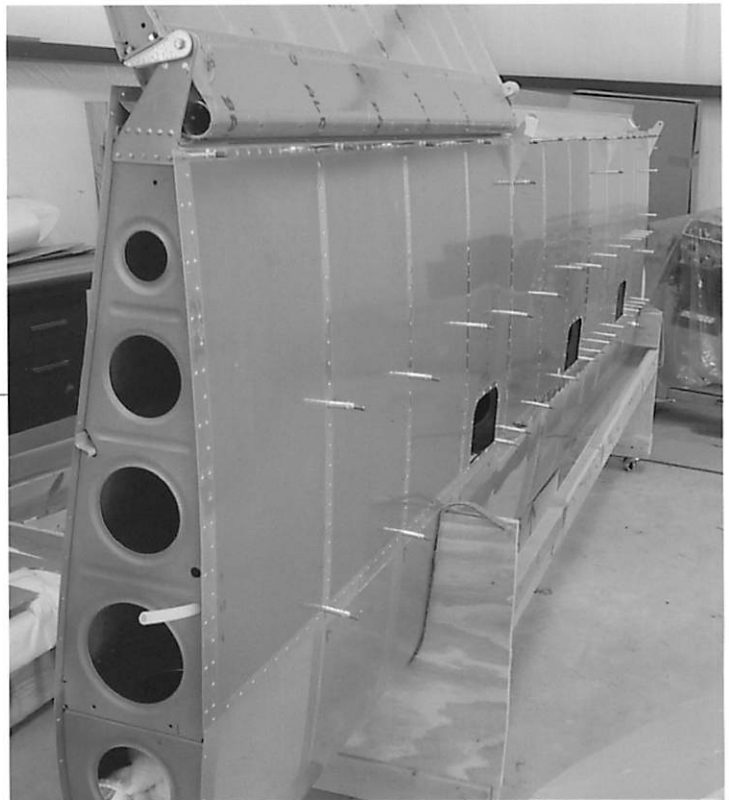
RV-9 Wing with aileron attached and bottom skin clecoed into position
