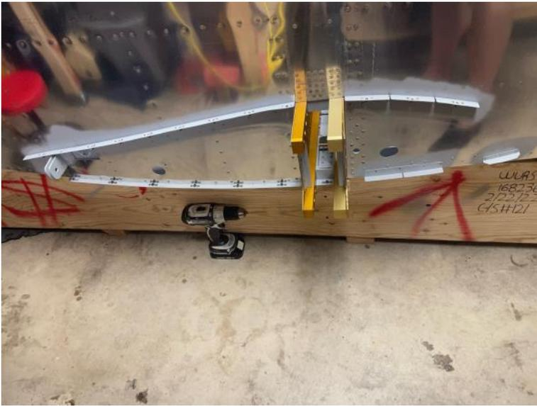
Next, I started building up the brace that also makes up the seat back adjustment rail. Bits of plastic were shaped to make guides for the adjustment arms.
