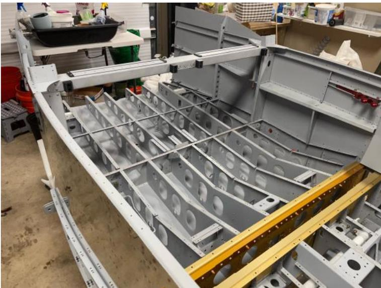
Finally, some gussets were fitted to both sides of the brace to build up the structure for the base of their roll bar. There were plenty of difficult rivets to buck in these tight spaces. Once it was done, I had a nice looking piece which is tying up this section of the plans.
