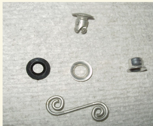
Dzus oval head stud, plastic retainer, short style aluminum retainer, full-size aluminum retainer, and "S" style receptacle spring. Note the "shoulder" undercut into the stud to accept the retainer. There is a stud without a shoulder which is often found on race cars.
