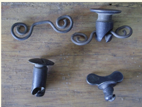
Dzus "U" style receptacle along with flush head, oval head, wing head studs
