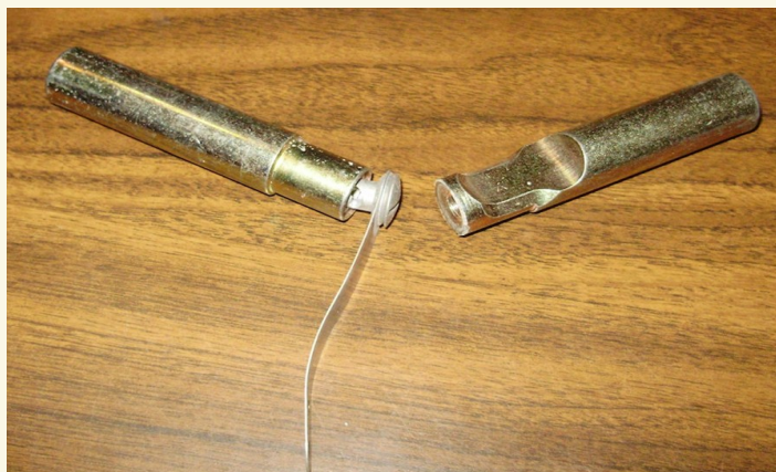
Dzus setting tool for #5 diameter studs. Here, a number 5 stud is inserted into a sheet metal fitting and a full size retainer has been swaged into the shoulder of the stud. The retainer is very flat and serves as a wearing surface. The odd cutout in the right-hand tool is for putting #5 studs into Beech Bonanza cowlings. Not shown is a handy Dzus driver tool which holds and turns the head of the stud better than a common screwdriver.
