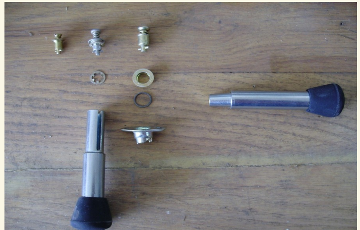
Camloc 2700, 2600, and 4000 studs, a star style retainer, a 4000 series grommet and retaining clip, and a typical receptacle. The right-hand tool is for placing the retaining ring onto the grommet. The tool at lower left is for placing a star retainer onto the body of a stud. Not shown are Camloc pliers which are nearly essential for inserting studs into sheet metal
