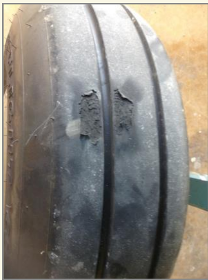
Reverted Rubber Due to Hard Braking on a Wet Runway
