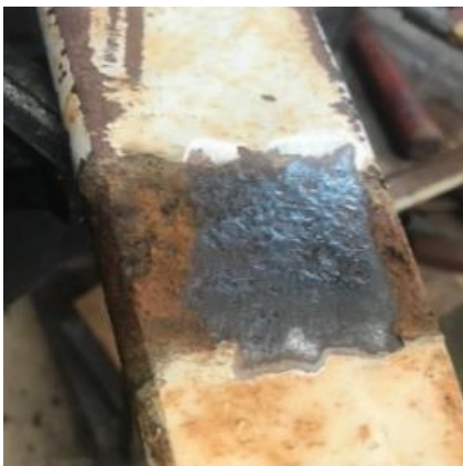
Photo 2: Rust under the step of a Cessna.
