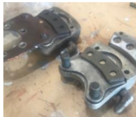
Photo 4a: Rusty vs clean Cleveland brake.
