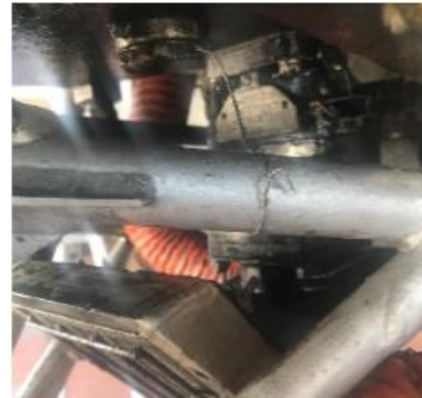
Photo 3: Safety wire around engine mount.
