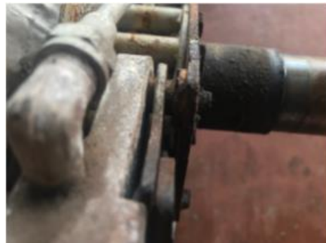
Photo 4: Rusty brake in situ.
