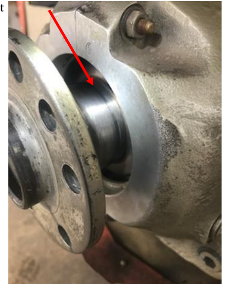
Photo 3: Groove in crankshaft
