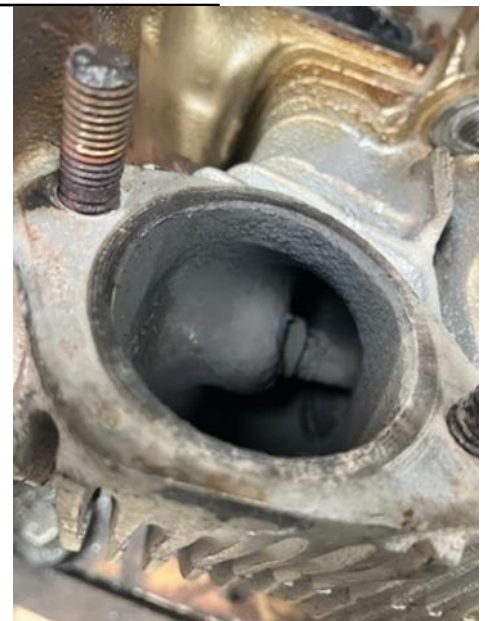
Photo 2: Carbon build up on an exhaust valve stem.
