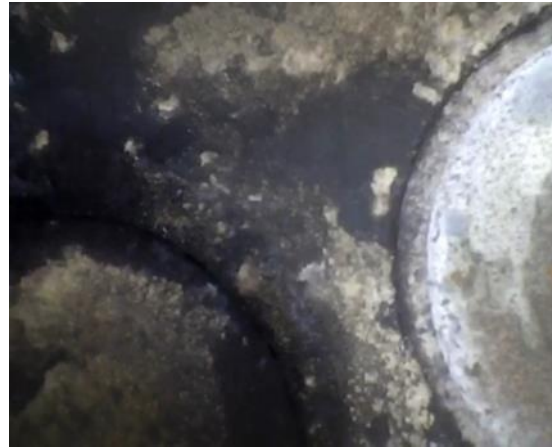
Photo 4: Borecope of the valves inside a cylinder
