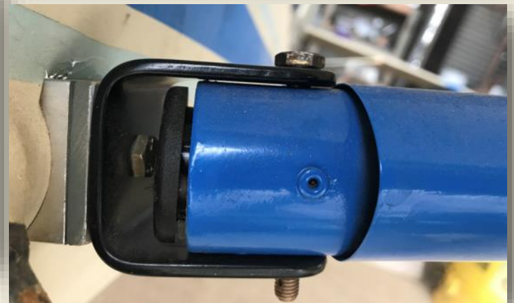
(this bracket has conformal shims on the left that brace the square bracket against the round tube on the left, which is under the aircraft fabric.)
