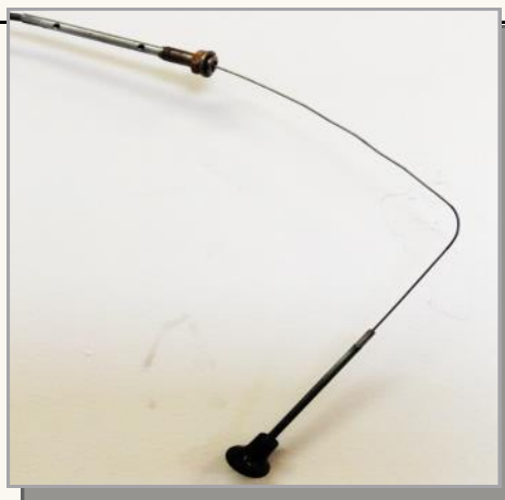
Photo 3: Modest pressure easily bent the push-pull wire at the blue spot.
