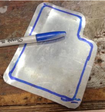
Photo 8: Guide line marked on heel plate blank.
