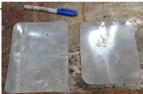
Photo 3: Two heel plate blanks cut out and ready for further fabrication
