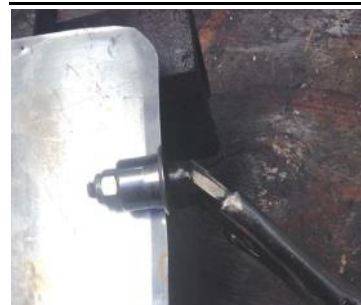
Photo 7: Edge rolling using a tool made from locking pliers.
