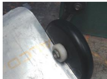
Photo 6: Edge rolling with a wheeled disk style tool.
