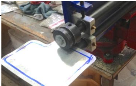
Photo 9: A blank in place ready to roll.
