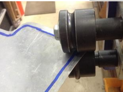
Photo 10: Beading around a corner.
