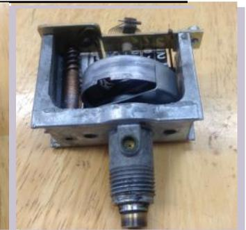
Photo 5: The Moving Parts of a Tachometer, Top View
