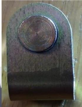
Photo 2: New Luscombe Rudder Hinge bracket and Pin.
