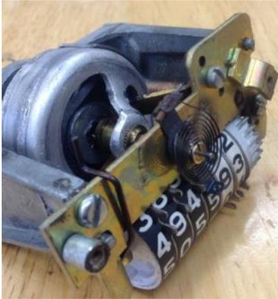
Photo 7: Front of Mechanism Showing the Calibrated Spring.
