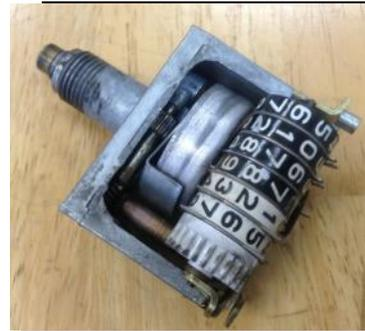
Photo 6: The Moving Parts of a Tachometer, Bottom View.
