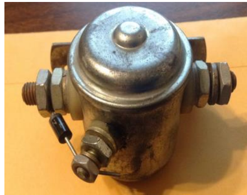
Photo 3: Diode properly oriented on a solenoid.
