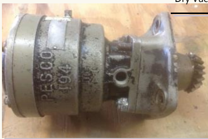
Wet Vacuum Pump
