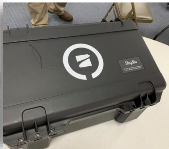
The symbol on the top of this carrying case serves as a landing pad designator that the drone can identify and return to.
