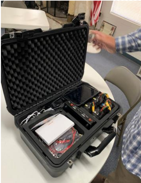
Other parts of a UAS include batteries, chargers, displays, controllers and more.
