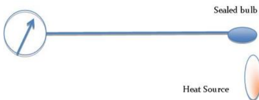
Figure 2: Schematic diagram of a capillary tube style temperature instrument.
