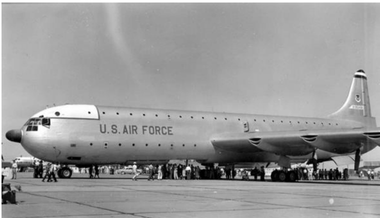
The radome was added in 1953 providing weather radar (www.nationalmuseum.af.mil)
