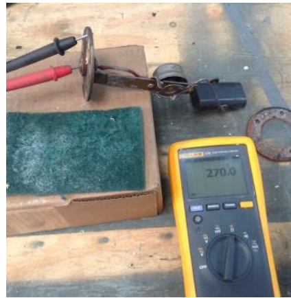
Photo 6: Fuel sender during bench check
