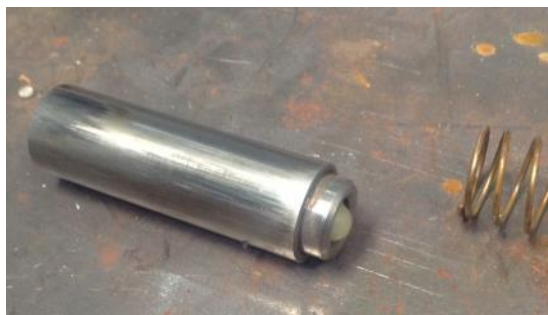
Photo 4: The silver cylinder is a shuttle with a one-way check valve built in.
