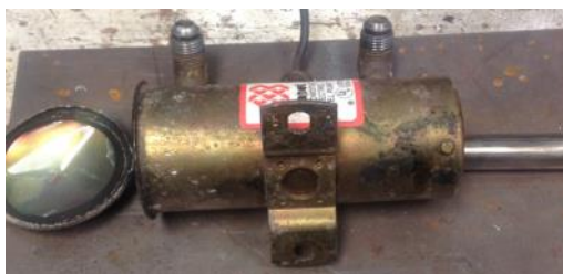
Photo 1: Facet fuel pump. Your Piper, Grumman, and sometimes Cessna have at least one of these
