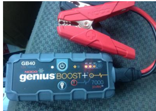
Photo 5: Commercially available battery booster.
