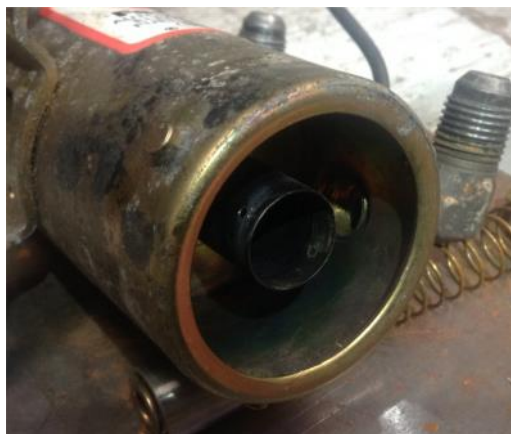
Photo 3: Inlet chamber of the pump. The filter basket goes here and the inner cylinder houses a shuttle valve.
