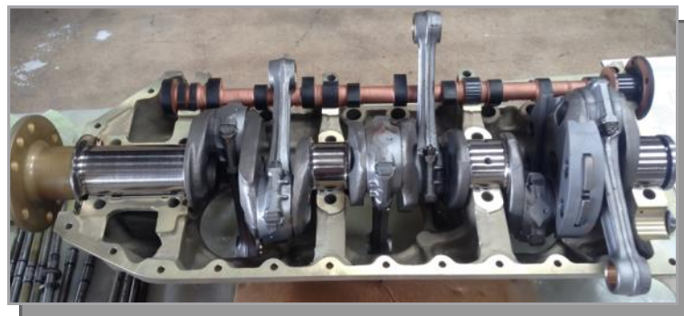
Photo 3: A Continental O-300 going back together. It may use the same cylinders and rods as the O-200, but inside the case is very different.
