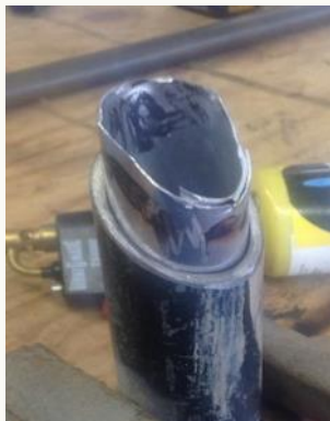
Here the black smudges are melted Tempil Stick and the gray scribble is unmelted Tempil Stick. Play with it awhile and you get the hang of it.
