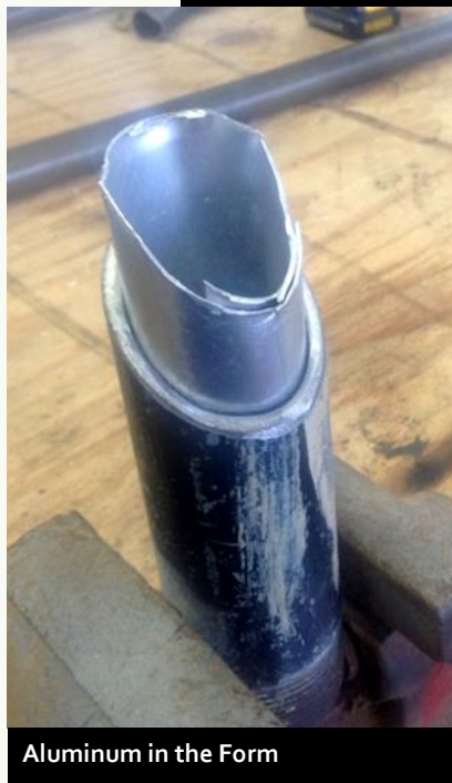
Rolled tube ready to form. Seamless tubing looks better, but rolled tube works fine. This is 5052 H14 .050 thick. If you don't know what that means then maybe you are not a sheet
