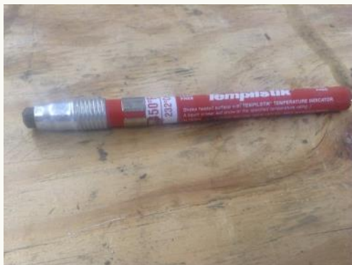
Here is my 450 Degree Tempil Stick. I have these in several temperatures. Buy them at your welding supply store.
