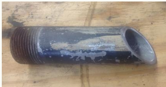
Blast Tube Form – this is one inch I.D. Smaller or larger forms are easy to make.
