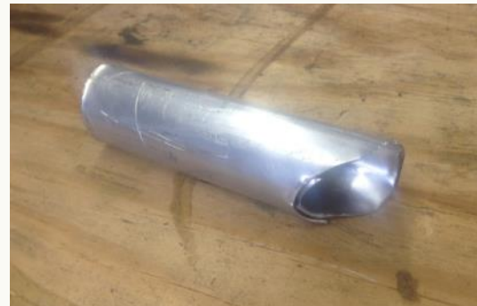
Rolled tube ready to form. Seamless tubing looks better, but rolled tube works fine. This is 5052 H14 .050 thick. If you don't know what that means then maybe you are not a sheet
