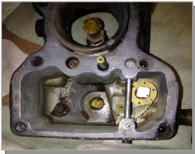
Stromberg Carburetor looking down into the opened float bowl.
