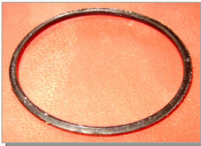
Gascolator O-ring Worn Into a Channel Shape.
