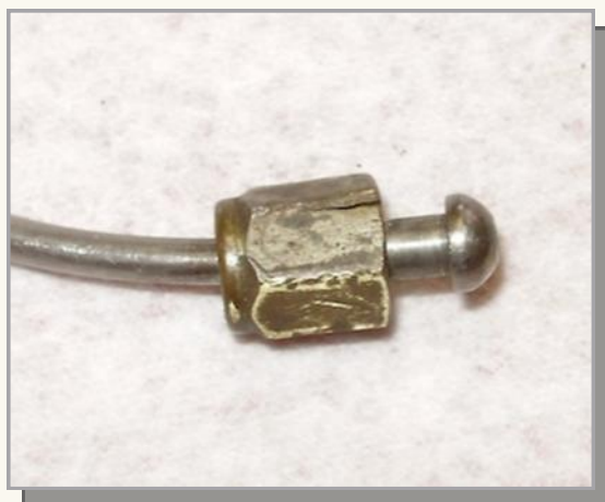
Cracked Brass Compression Nut on a Fuel Injector Line.
