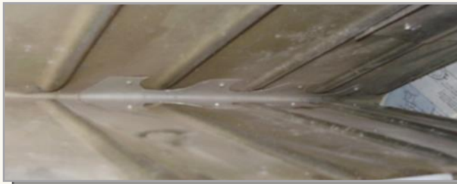
Repair Patch Inside a PA-28 Rudder.
